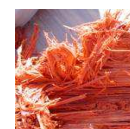
Dark stringy rot - DSR Has a coarse stringy texture, ranging from light brown through to dark reddish-brown. Appears to consist of long, stringy, wool-like fibres.
