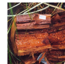
Mudguts - MUD Has a characteristic clay-like consistency, and appears devoid of recognisable wood fibres. Mostly occurs in the inner heartwood, sometimes associated with a hollow, but also occurs in localised patches in outer heartwood. Often found adjacent to red-brown blocky fibrous rot.
