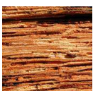
Combination pocket dark rot - CPD Characterised by irregularly spaced 5-20 mm elliptical pockets. These are generally empty but occasionally filled with white gelatinous or crystalline material (cellulose). The wood breaks into regular blocks, and the wood in between the pockets is soft. It is light brown to red-brown.
