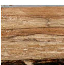
Small pocket rot - SPR Characterised by 2-5 mm elliptical pockets, which are usually empty but occasionally filled with white gelatinous or crystalline material (cellulose). Pockets are separated by thin areas of seemingly intact wood. Can range from light tan to dark reddish-brown. Often has black 'zone' lines.
