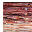
Pale pocket rot - PPR Characterised by 5 – 20 mm regular round to elliptical pockets, which are either empty or are filled with white gelatinous or crystalline material (cellulose), or may be lined with white or yellow mycelium. Pockets are separated by thin areas of seemingly intact wood. Mostly occurs in a log's outer regions.
