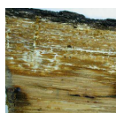
Fibrous surface rot - FSR Occurs in the top 1 – 5 cm of the log surface layer but can extend into the outer heartwood. Has a soft stringy texture, ranging from grey-white to straw or brown. Seems to consist of numerous minute irregular pockets, speckled with soft bleached fibres.
