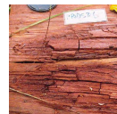
Dark blocky fibrous rot - DBF Characterised by brittle wood that breaks off in regular blocks and can be crumbled to powder by hand. Tan or light brown. Consistently very dry. Sheets of mycelium, with a chamois-like texture, progress along the rays.
