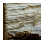
Pale spongy rot - PSP Characterised by continuous long, spongy, wool-like, bleached fibres. Can range from white to a straw-yellow. Has a very soft texture and appears to have a very low density.
