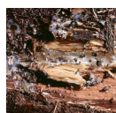
Jelly surface rot - JSR Characterised by large (> 50 mm) irregular pockets which may be empty or filled with white, soft, very wet, gelatinous or crystalline material. Black 'zone' lines demarcate the pockets. Rhizomorphs also present.
